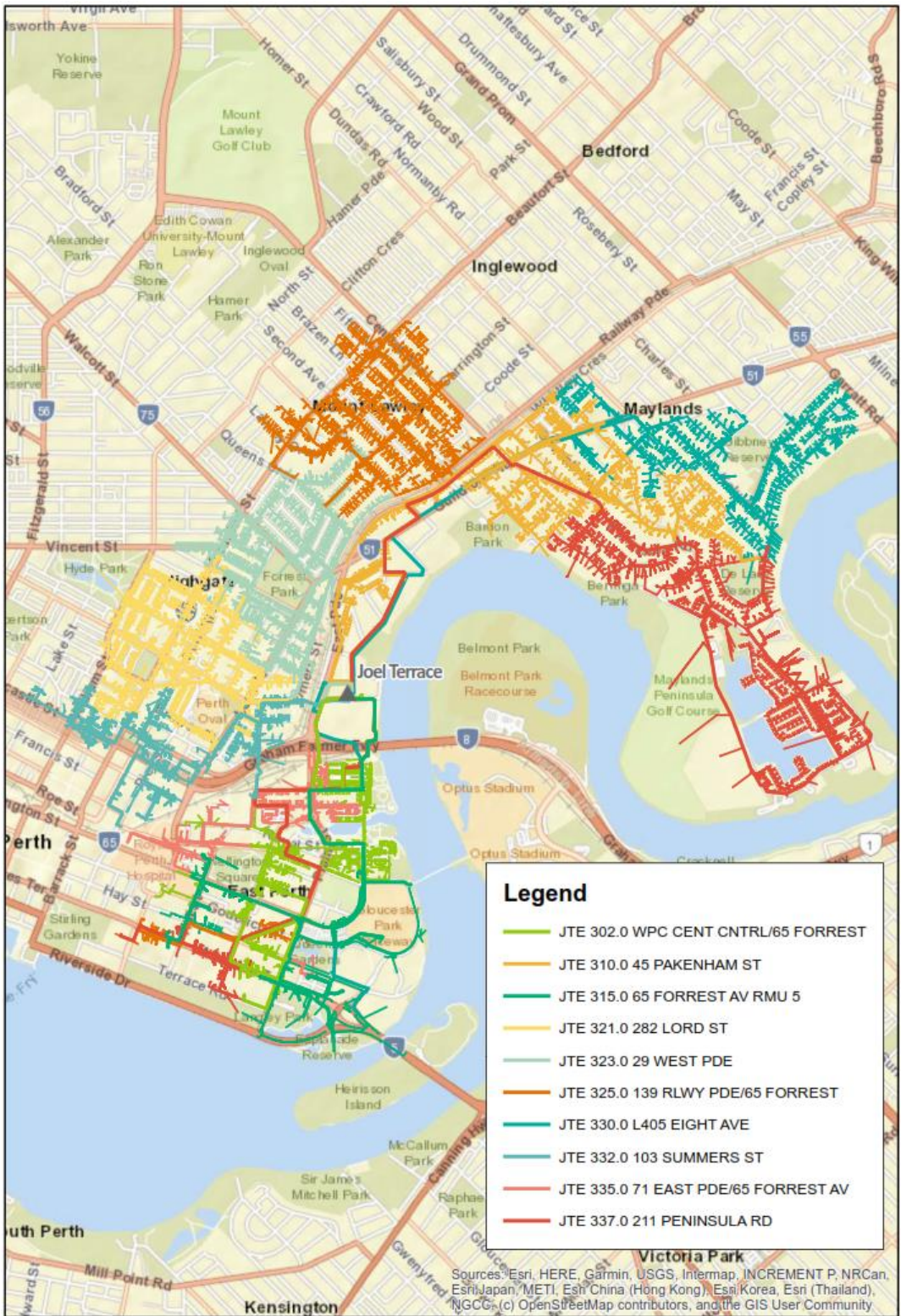
Figure 3.3: Geographical distribution of Joel Terrace high utilisation feeders (JTE 302R, JTE 310, JTE 315F, JTE 321F, JTE 323F, JTE 325F, JTE 330F, JTE 332F, JTE 335F and JTE 337F) 22
